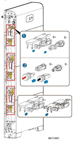
Figure 5-3 DC power cable connection inside the battery
