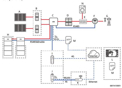
**Figure 3-1** Grid-tied ESS networking diagram (dashed boxes indicate optional components)
