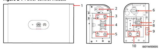
(1) Power control module (2) Black start switch module (3) Battery terminals (BAT+/BAT-)
