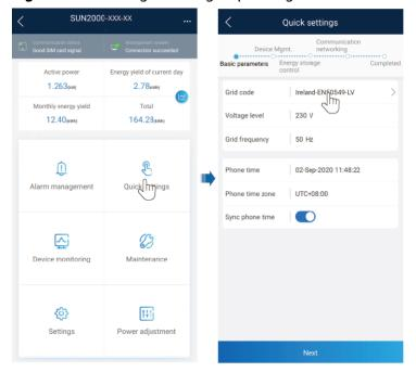
Figure 3-15 Setting the off-grid power grid code
