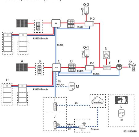
**Figure 3-12** Inverter (with batteries) + inverter (with batteries) (dashed boxes indicate optional components)
