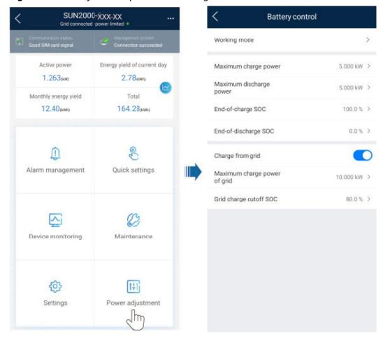
Figure 6-6 Battery control parameter setting
