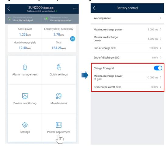
Figure 3-7 Battery control parameter setting
