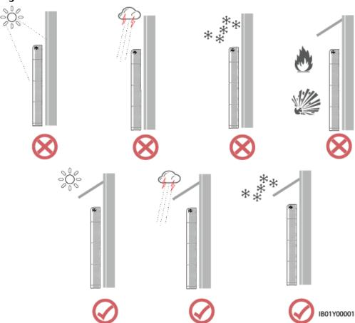
Figure 1-1 Installation environment
