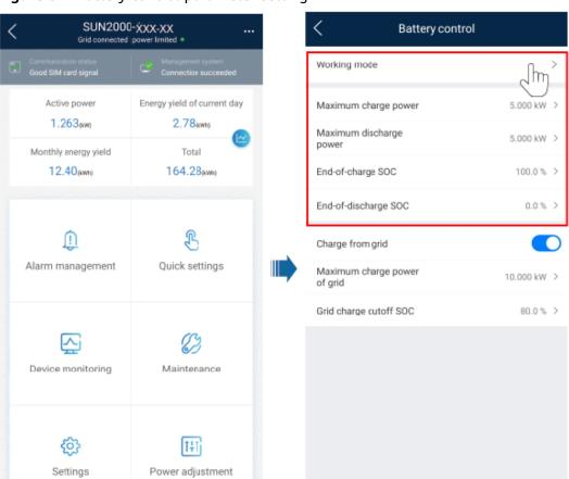
Figure 3-4 Battery control parameter setting
