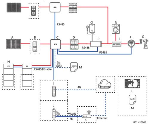
**Figure 3-11** Inverter (with batteries) + inverter (without batteries) (dashed boxes indicate optional components)
