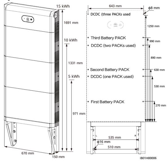
Figure 4-7 Wall-mounted installation dimensions
