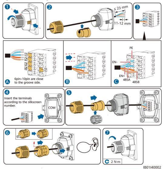
Figure 5-14 Connecting inverter terminals
