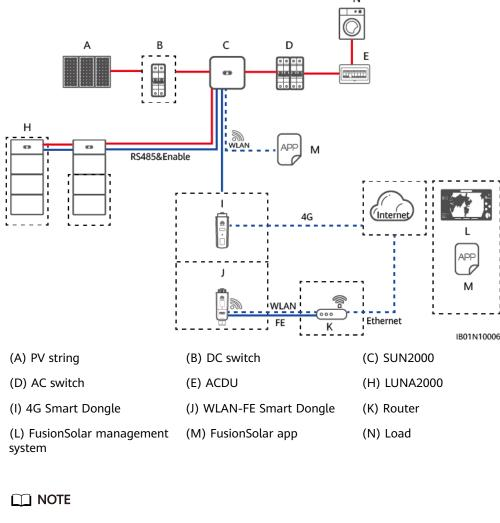
Figure 3-14 Off-grid ESS (dashed boxes indicate optional components)
