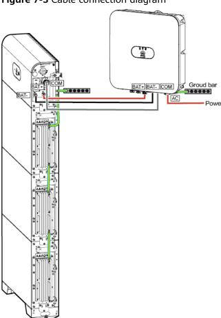
Figure 7-3 Cable connection diagram
