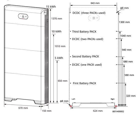
Figure 4-2 Floor-mounted installation dimensions
