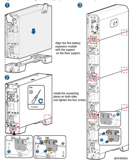
Figure 4-5 Installing the battery expansion modules and power control module
