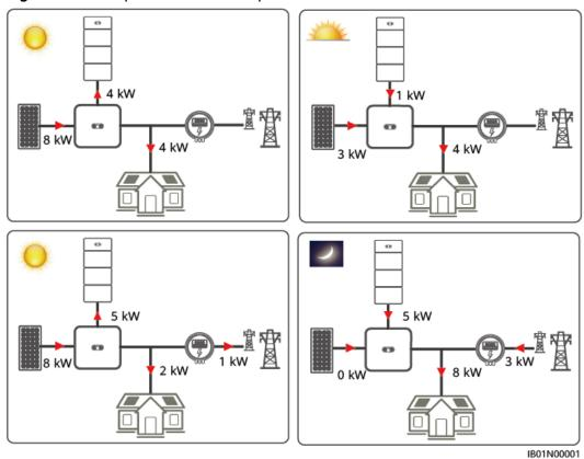
Figure 3-5 Example of Self-Consumption
