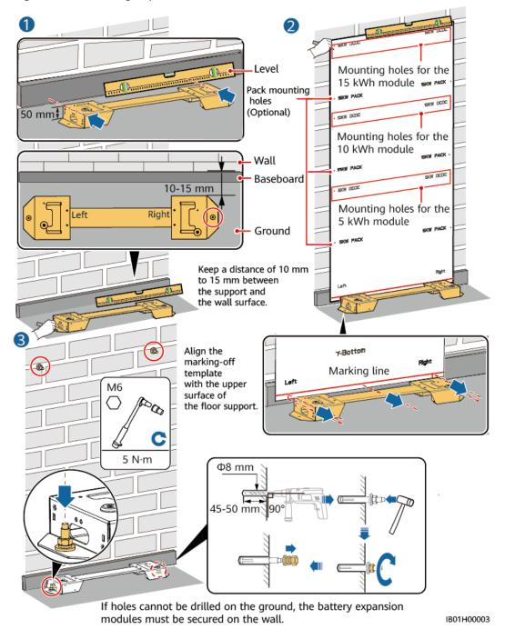
Figure 4-4 Installing expansion bolts
