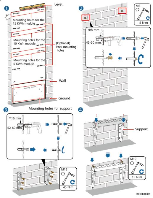
Figure 4-8 Wall-mounted installation
