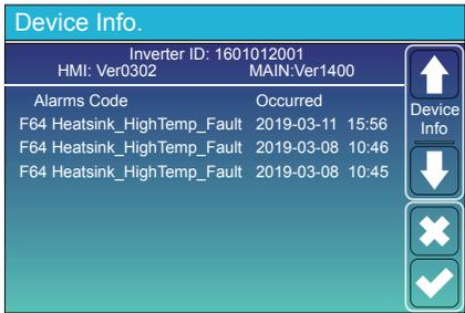
This page shows the Inverter ID, Inverter version and alarm codes.
