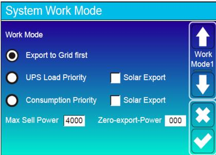
**Export to Grid First** - When the inverter is grid connected any excess energy will be exported to the grid.
