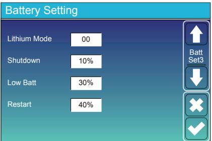
**Off-Grid Battery Setup**
