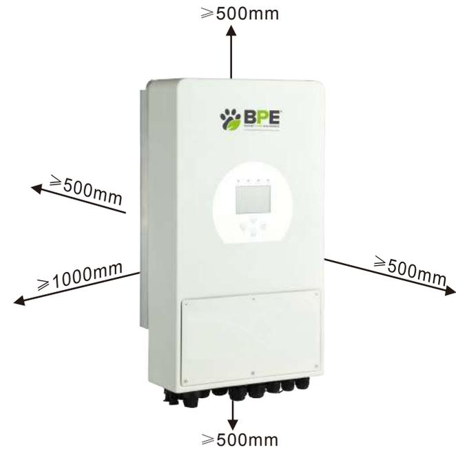
For proper air circulation to dissipate heat, allow a clearance of approx. 50cm to the side, approx. 50cm above and below the unit and 100cm to the front.
