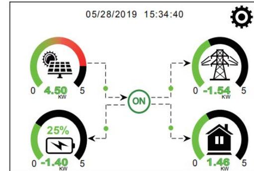
1. The icon in the center of the home screen indicates that the system is in Normal operation. If it displays "comm./F01~F64", this means the inverter has communication errors or other errors, the error message will be displayed under this icon (F01-F64 errors, detailed error info can be viewed in the System Alarms menu).
